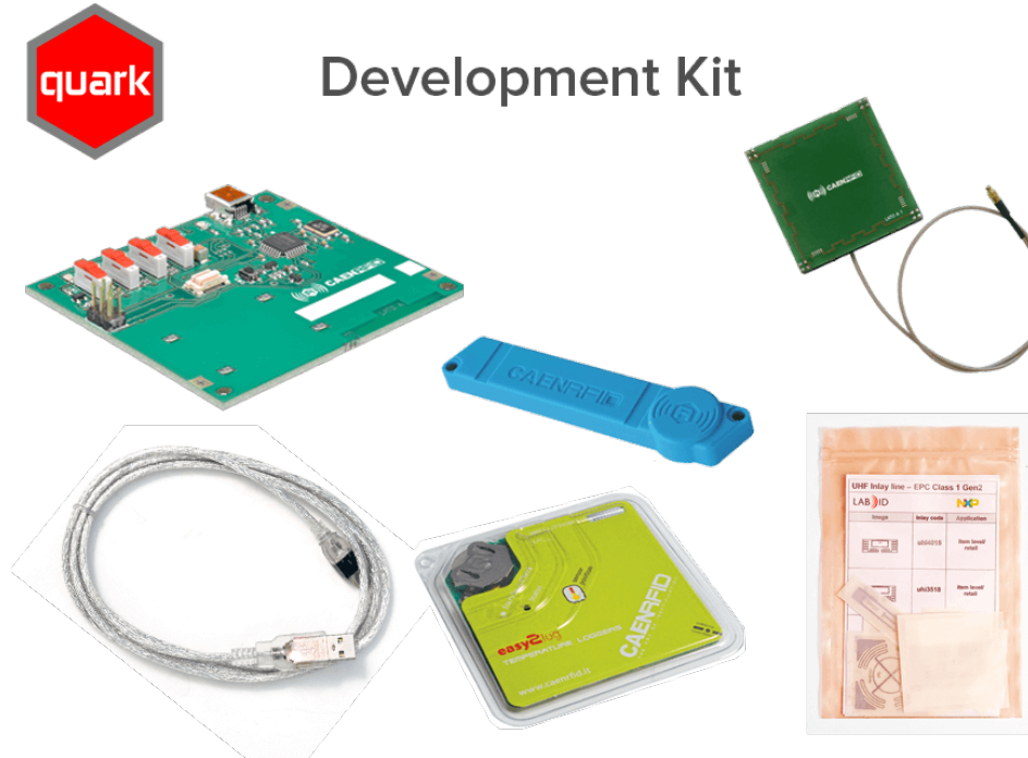
Fig. 1.3: R1230CBDK - Development kit with evaluation board, antenna and tags
