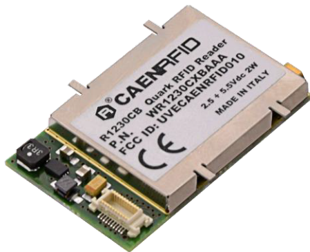
Fig. 1.1: Quark R1230CB OEM UHF Multiregional compact reader
